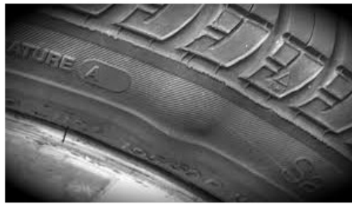
Bulges, tyre is illegal
